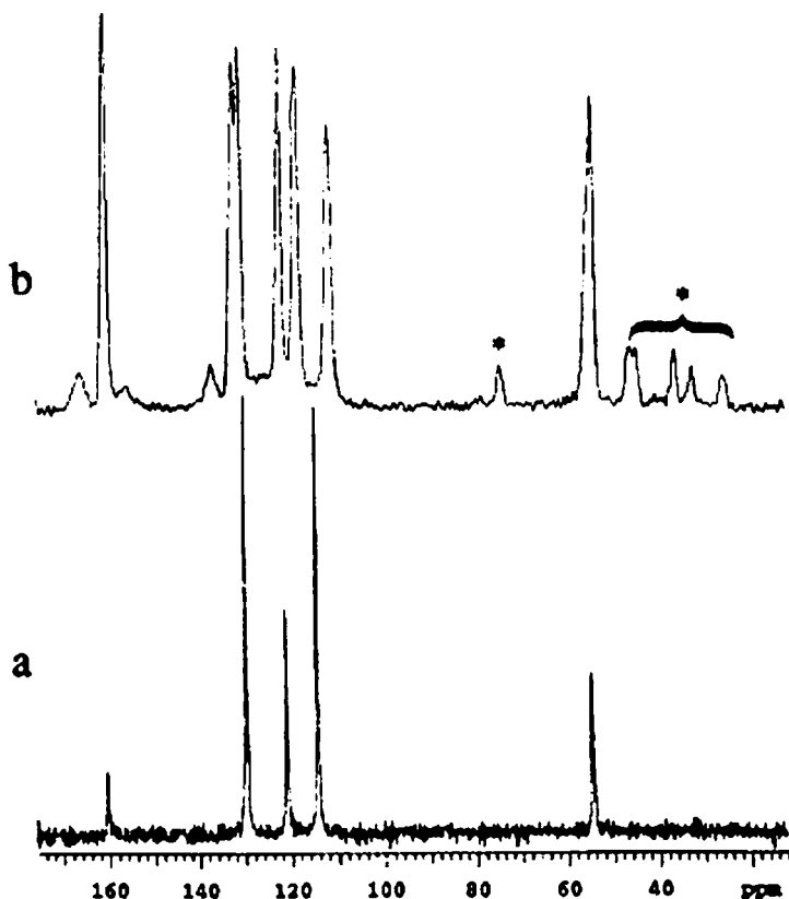
Fig. 1. High resolution spectra of anisole at (a) room temperature liquid and (b) MAS spectrum at 180 K showing the splitting of the aromatic carbons upon freezing out the motion of the methoxy group. Peaks marked with asterisks are MAS side bands. (Reproduced with permission from ref. 18.)
